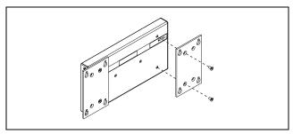
Figure 9. Compact FieldPoint Horizontal Panel-Mount Kit with cFP-BP-4
